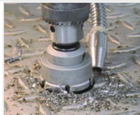
Drilling structured sheet metals
