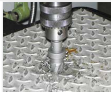
Drilling structured sheet metals
