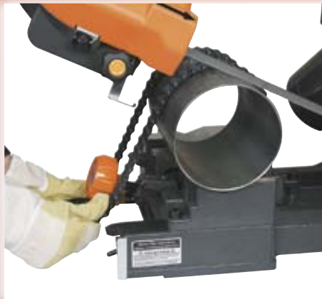
Changeable chain vice in action RBX 180 HV
