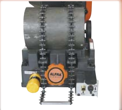
Clamped pipe in chain vice RBX 180 HV
