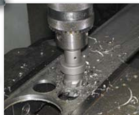
Drilling flat steels
