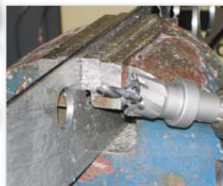
Free-hand drilling up to Ø 30 mm
